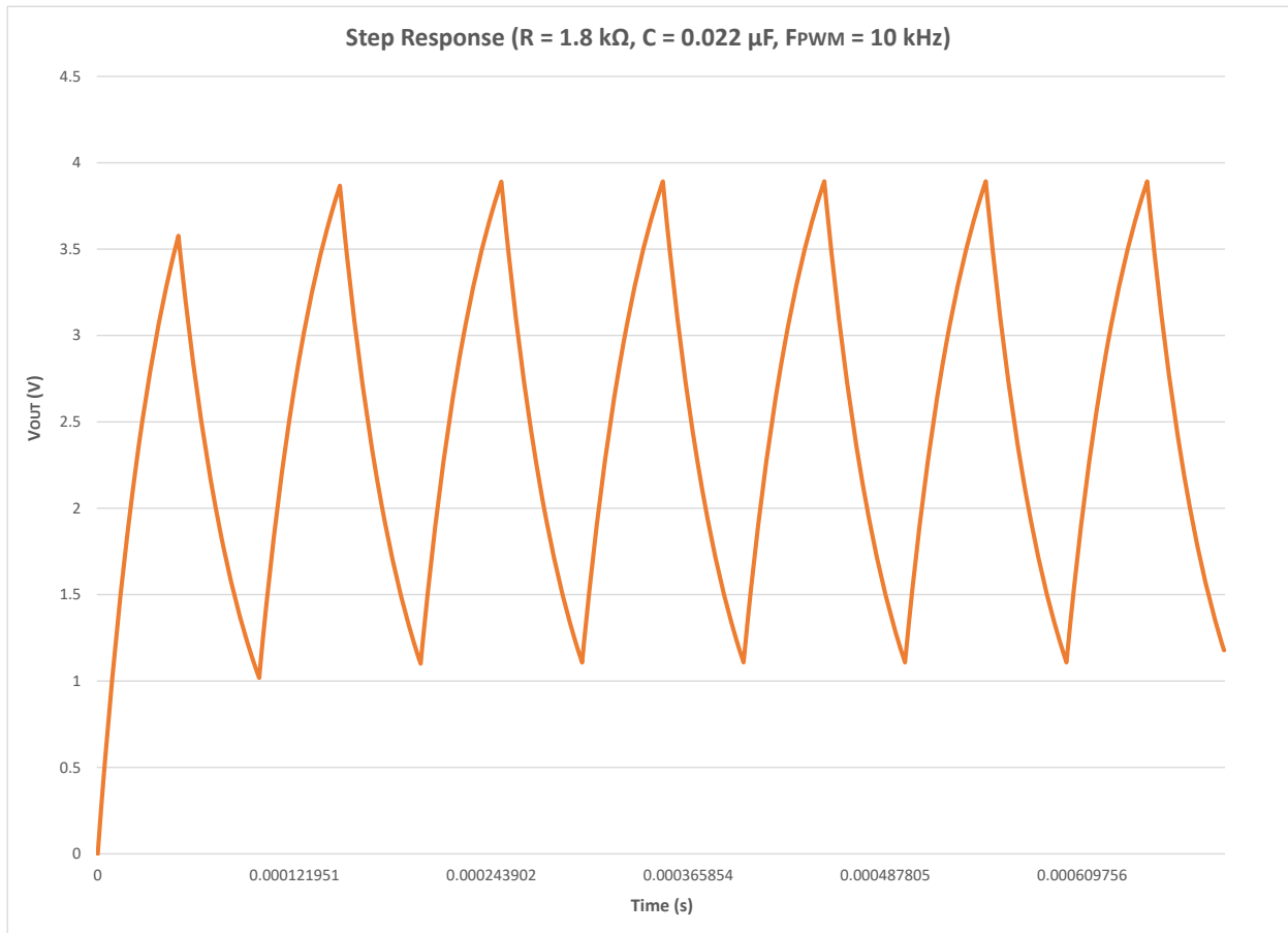
Figure 2-9. Step Response ( R = 1.8\text{ k}\Omega , C = 0.022\text{ }\mu\text{F} , F_{\text{PWM}} = 10\text{ kHz} )
